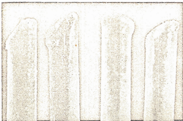
Fig. 13. Representative bristles selected from a .012" bristle brush, serrated trim, that had been used daily, generally with prepared chalk, for more than four months. Note that the sharp rough edges have finally been smoothed off considerably, thereby lessening their harmfulness
